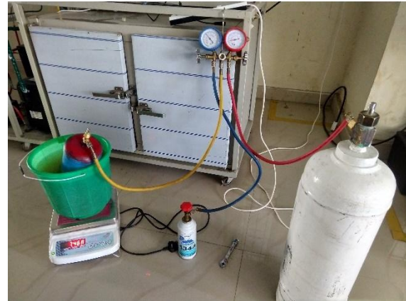
Fig. Gas Mixing Process
